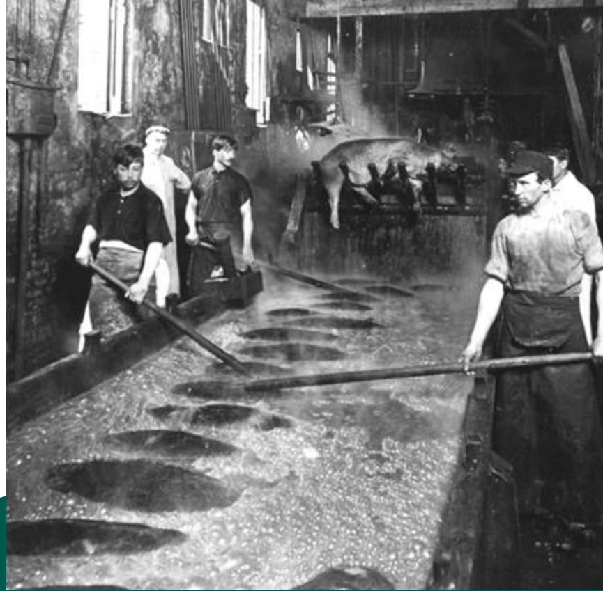
Boiling vats used to prepare hogs for hair removal, circa 1890
